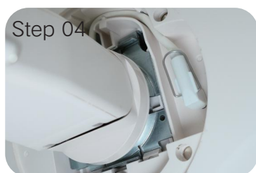
Step 04 Connect the screen to power
