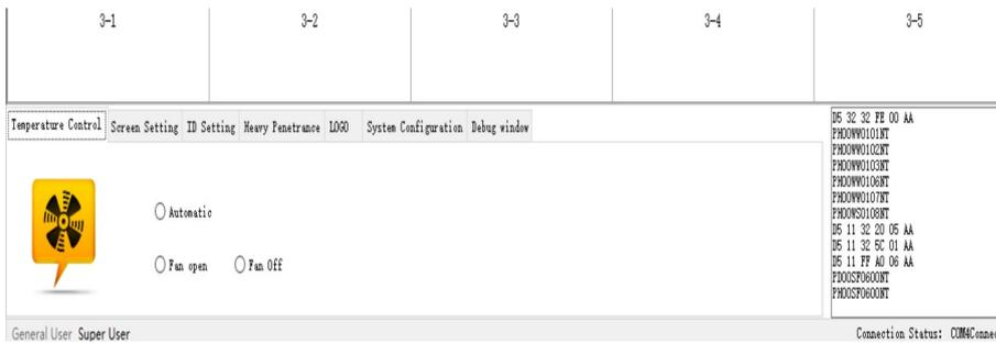
Temperature fan control, the default is "Auto" mode: > 45 degrees open, < 40 degrees off; The other is normally open, normally closed, and other modes can be set manually for customers to choose.
