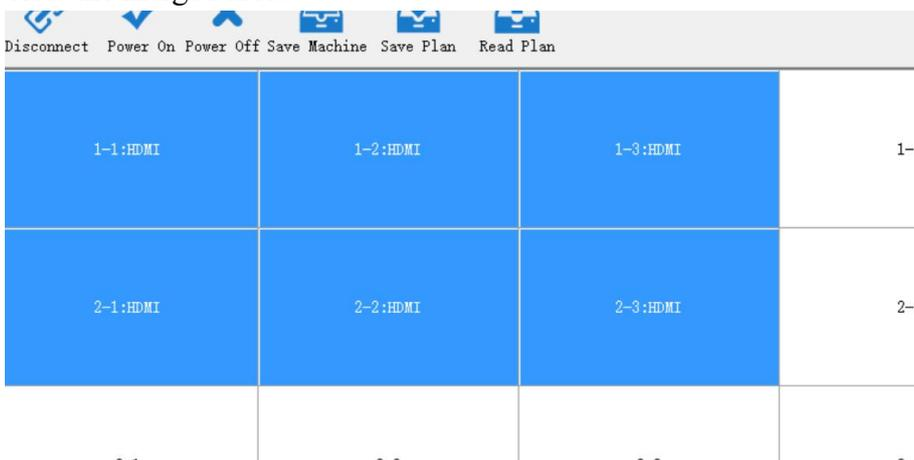
In the above case, 3X5 matrix system, we need to coordinate (1,1) - (2,3) region spliced into a 2X3 large screen display.
